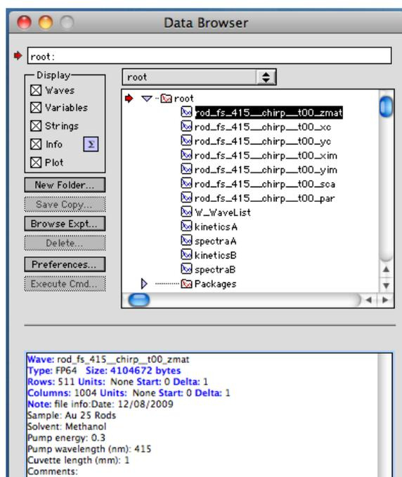
The footer information in the original file (beginning with “file info”) is stored in *filename\_zmat* as an Igor Note. This information can be viewed directly from the Data Browser by highlighting the appropriate wave. Alternatively, it viewed from any plot, by holding down Command-Option-Control (Mac) or SHIFT+F1 (Windows) and clicking on the graph.
